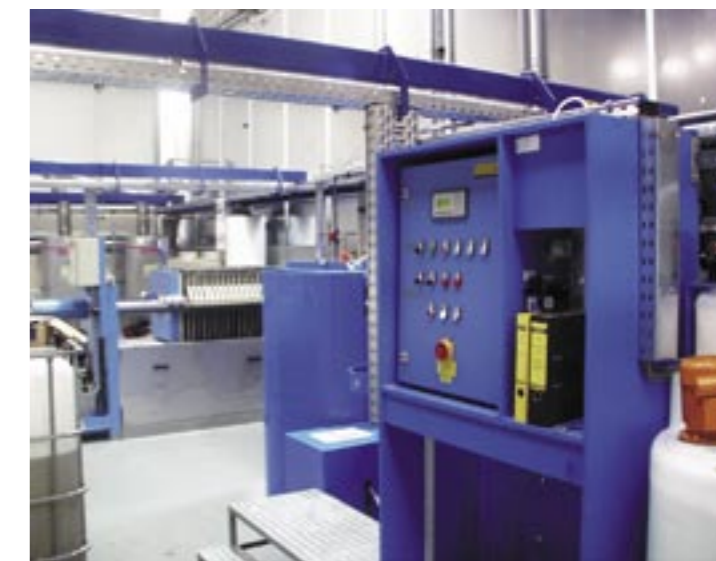
ADF-flotation with chamber filter-press for surface dewatering at storage areas or transshipment spaces of discarded metal with adherence of emulsion.
